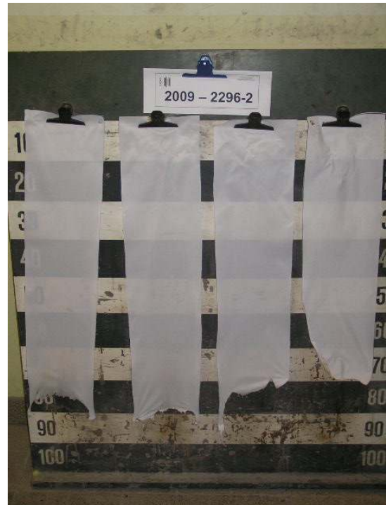
Appearance of sample B after the "Brandschacht" test
